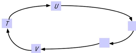
transactions is indirect, via a dependency on objects. The diagram on the right shows the objects held by and waited for by transactions  $T$  and  $U$ . As each transaction can wait for only one object, the objects can be omitted from the wait-for graph – leaving the simple graph on the left.
