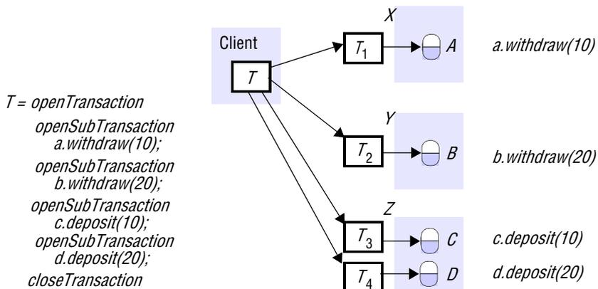
**Figure 17.3** A distributed banking transaction
