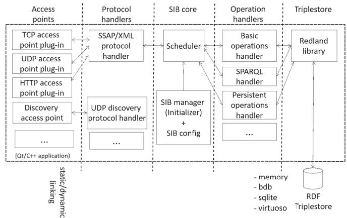
Fig. 4. The plug-ins based architecture of CuteSIB
