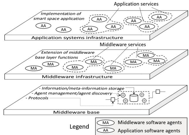
Fig. 1. Infrastructure multi-layer model of semantic-oriented middleware
