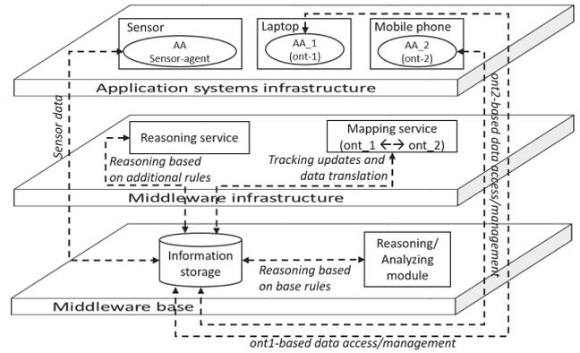
Fig. 3. Implementation of semantic interoperability requirement based on the infrastructure multi-layer model of semantic-oriented middleware
