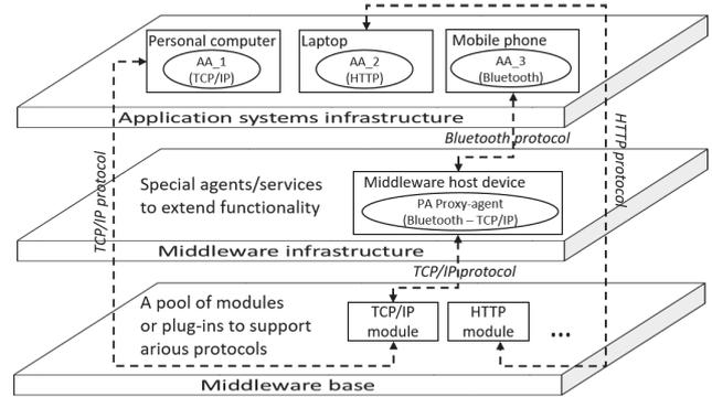
Fig. 2. Implementation of extensibility requirement based on the infrastructure multi-layer model of semantic-oriented middleware
